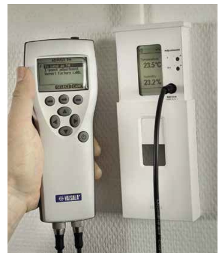
On-site calibration of a HMW90 humidity transmitter with a HM70 hand-held meter.
