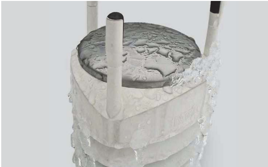
The WXT520 has an automatic control circuit that switches the heating on at low temperatures.
