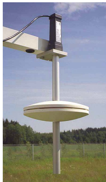
The SPH10/20 is easy to install and connect. In the picture, a SPH10 is connected to a PTB210 barometer.
