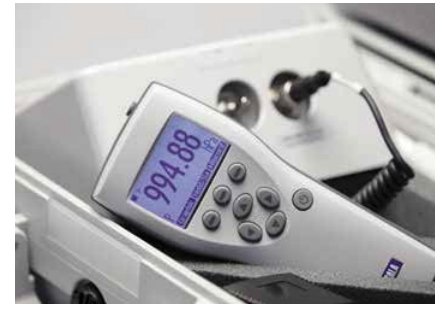
The MI70 hand-held indicator displaying the prevailing pressure in hPa
